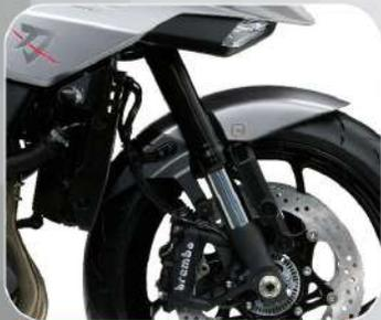
Fully adjustable, inverted front forks
