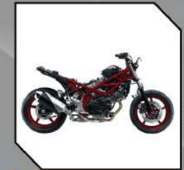
Truss Pipe Frame
