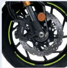
Solid grip tires Radial mounted four-piston opposed front calipers
